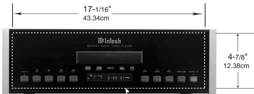
MVP861 Front Panel Custom Cabinet Cutout
